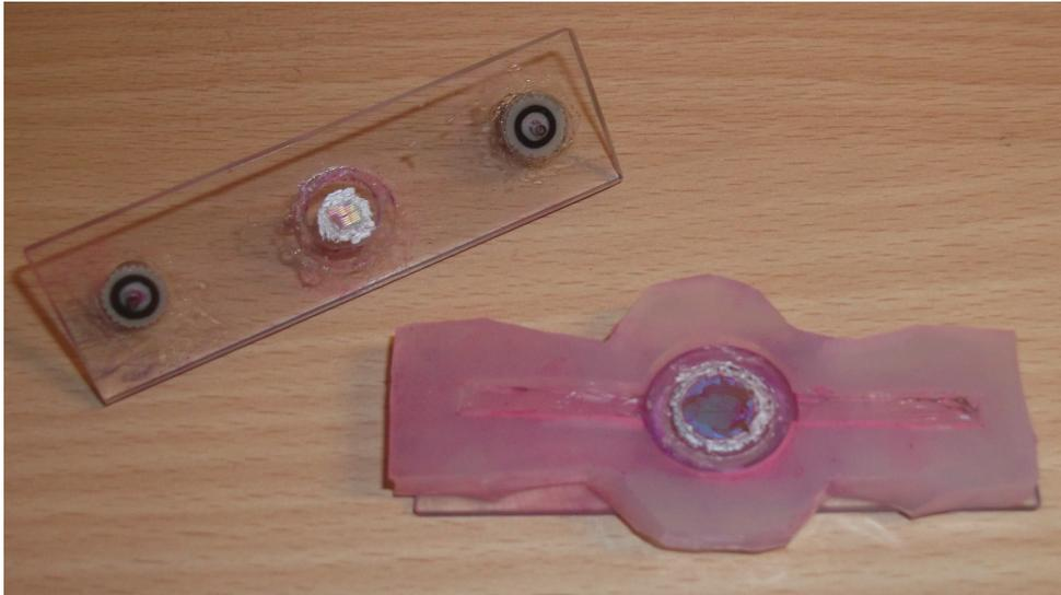
**Figure 11:** Photograph of flow cell. The diminutive size of the featured substrate visible in the middle of the top plate can be appreciated. The rubber seal has been fitted over the plinth
