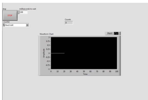
Figure 3.1.4 Print screen of the SPAD counter front panel in Labview. This is the user interface, with a waveform chart to display photon count rate
