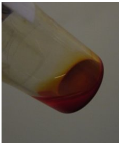
FIGURE G.2: The agglomeration of eFluor ® 650 nm nanocrystals at 4°C.
